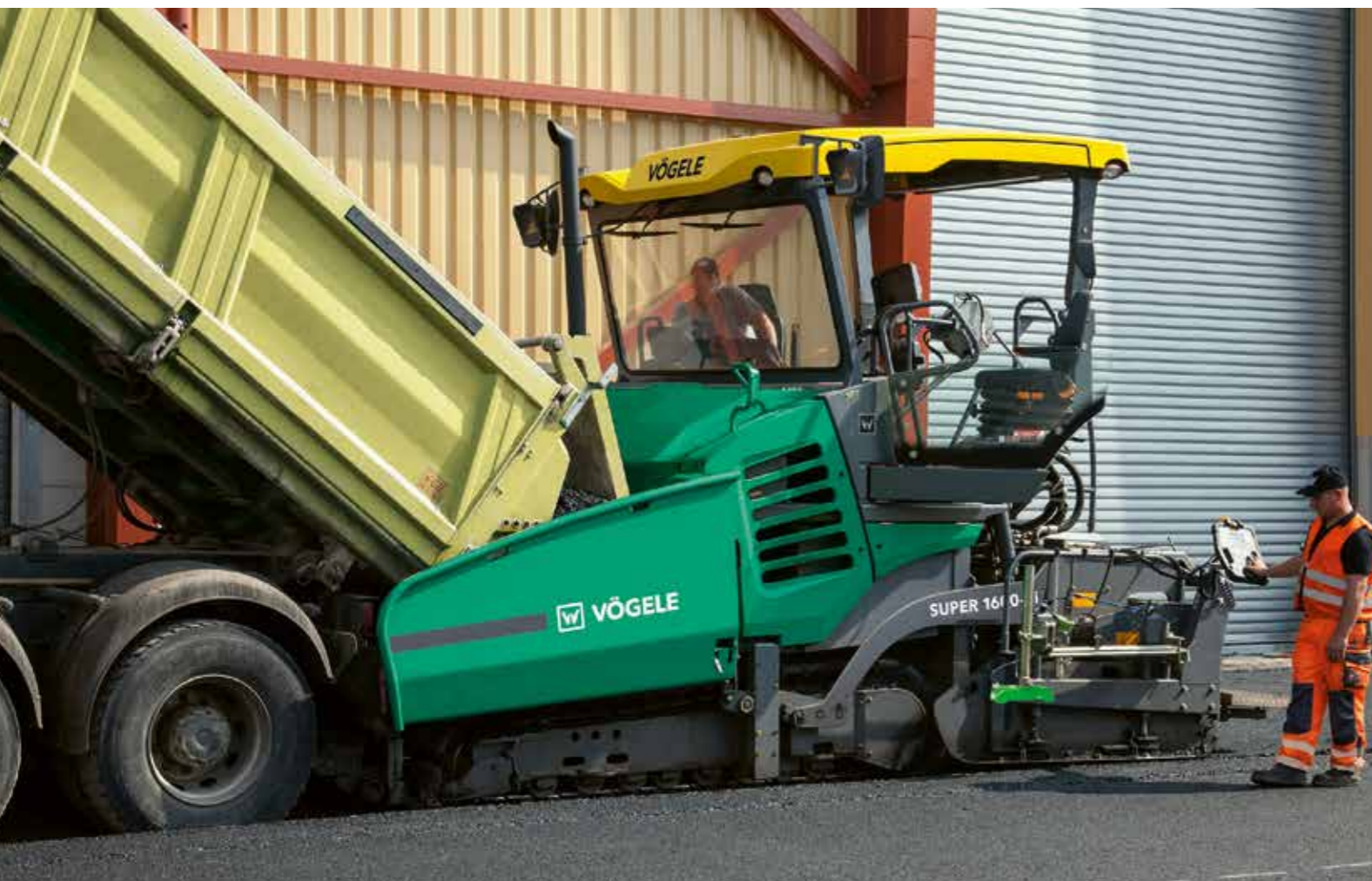
PaveDock sprung push-bar reliably absorbs any jolts from feed vehicles.
