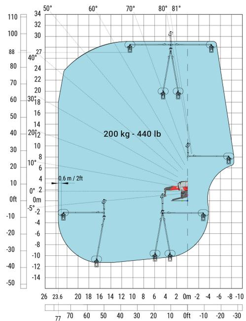
Machine on lowered stabilisers with extensible jib with winch (Metric)
