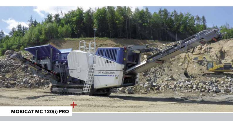
The MOBICAT MC 120(i) PRO, the first jaw crusher in the PRO line, is used for precrushing almost all types of natural stone. The jaw crusher is extremely robust and impresses with its low-maintenance operation. The machine therefore guarantees high production outputs.
